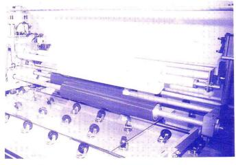
The CLM-1300 GL is useful device to make glass clean prior to Laminating and Printing. The operation is entirely simple ... everybody
